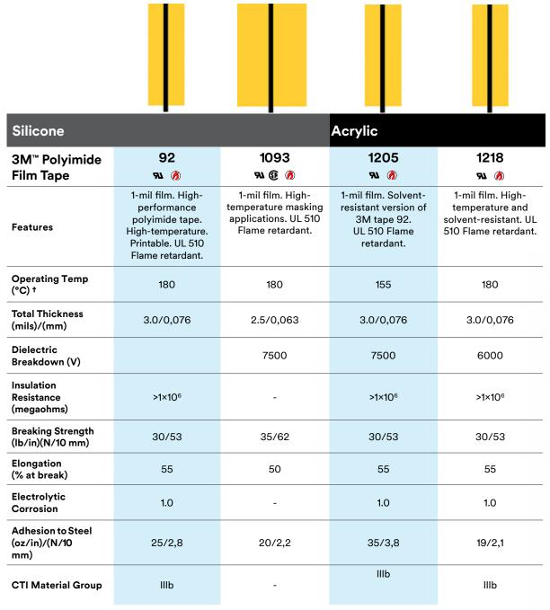
Operating temperature is equivalent to UL Recognition temperature where applicable (See page 16).
