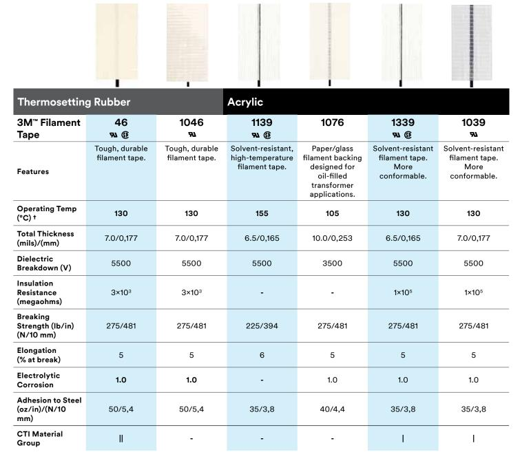
Operating temperature is equivalent to UL Recognition temperature where applicable (See page 16).
