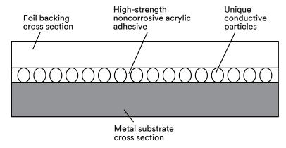
Figure 2 Embossed Backing with "Through-the-Adhesive" Contact
